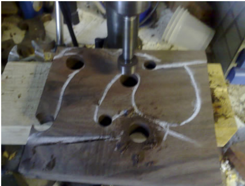
Drill out the corners.
