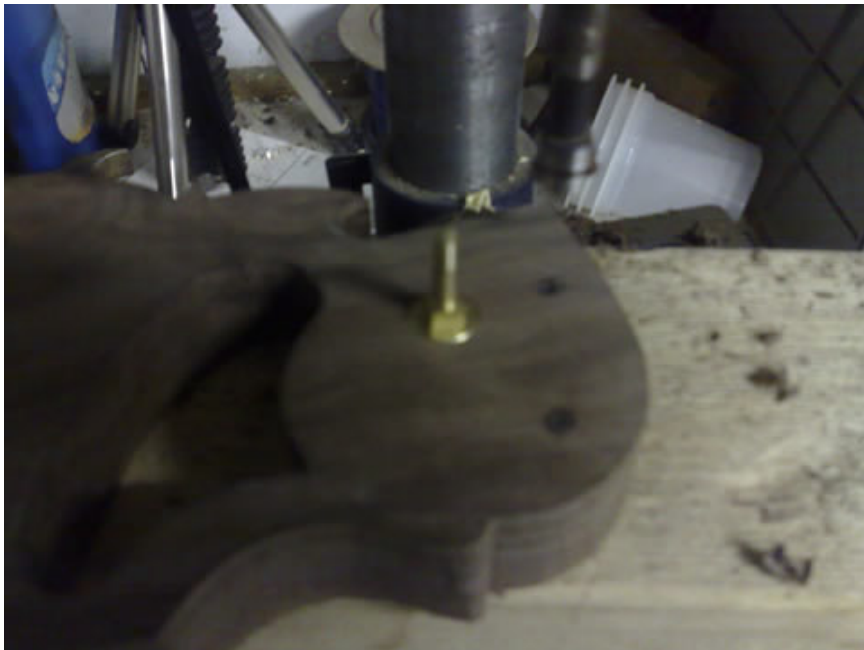
Drill screw head recesses with a forstner bit
