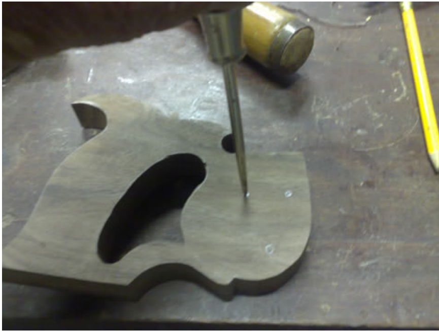
Mark the holes
