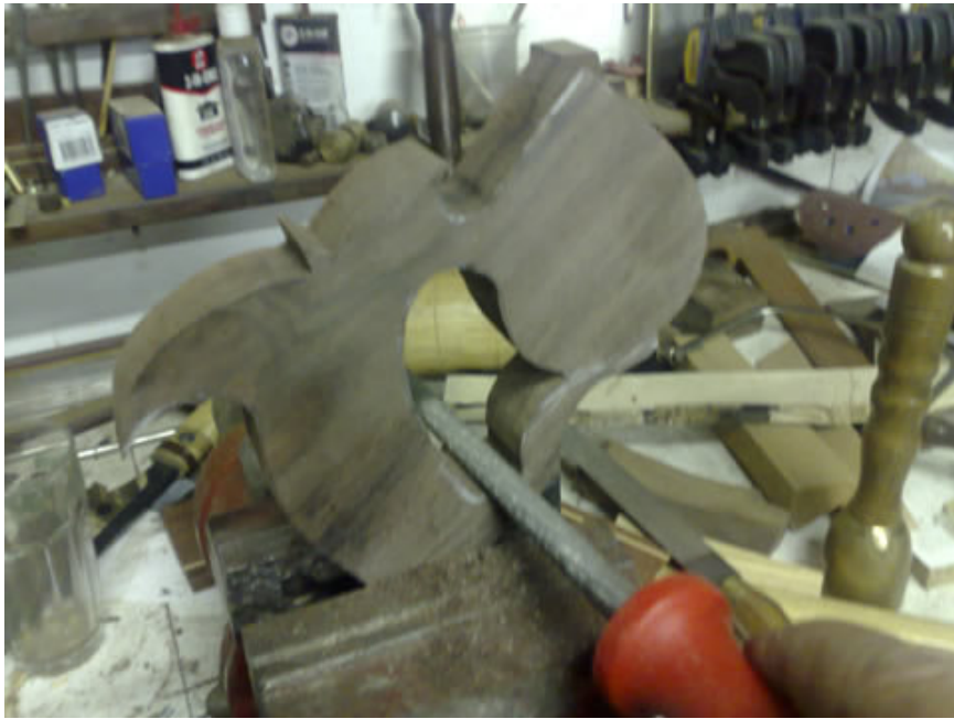
For tighter curves a round file works just fine.
