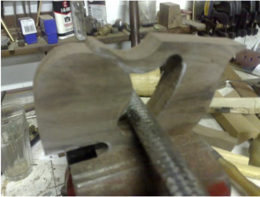
Microplanes cut fast and leave a pretty good finish.
